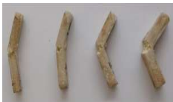
Figure 5. Specimen After Charpy Impact Testing
