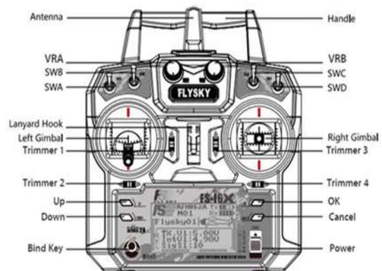
**Figure 4.3** Flysky i6 Transmitter Schema
