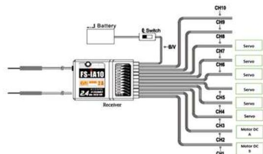
**Figure 4.4** Schematic 2.4Ghz 10CH Flysky Receiver Circuit
