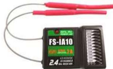
Figure 2.7 Flysky Receiver Module 16
