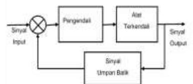
**Figure 2.2** Diagram of a Closed Network Control System
