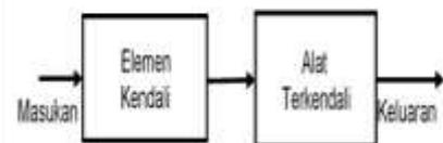
**Figure 2.1** Diagram of an Open Network Control System
