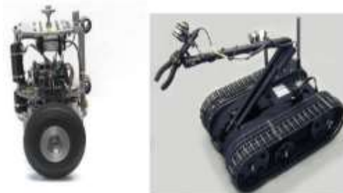
Figure 2. 2 Two-wheeled robot (a) and a Caterpillar wheeled robot (b) (Source: http://www.eprints.undips.ac.id.com )
