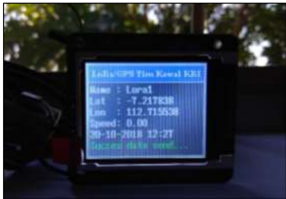
Figure 24 Testing on the KMR-1.8 SPI TFT display
