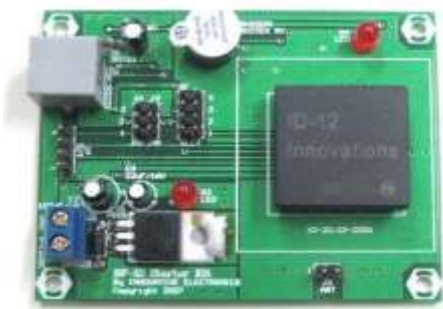
Gambar 2 Reader RFID stater kit ID-12 LA.
