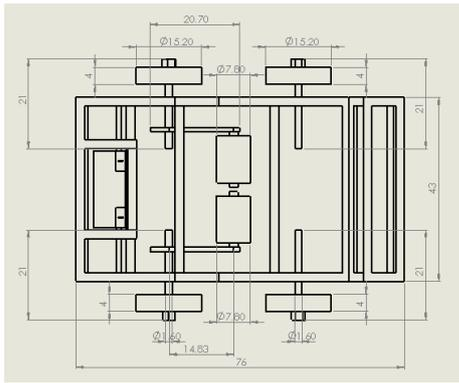
**Figure 3.** Figure 2 D TGV top view (in cm)
