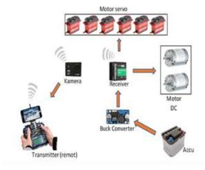
Figure 4.1 Toolkit Schema (Source: Self-processed Results)
