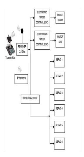
Figure 3.2 Block Prototype diagram of a robot arm
