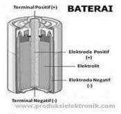
Figure 2.10 Batteries (Source: www.Productionelektron.com)
