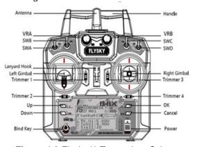
**Figure 4.3** Flysky i6 Transmitter Schema (Source: https://robu.in/product/flysky)
