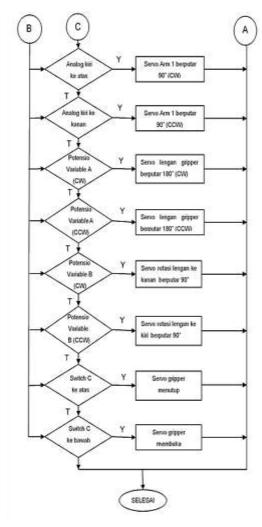
Figure 3.3 Flowchart Prototype Base and Robot Arm
