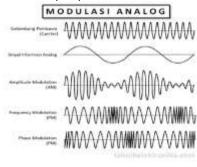
**Figure 2.4** Analog Modulation (Source:
