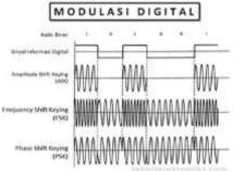
Figure 2.5 Digital Modulation
