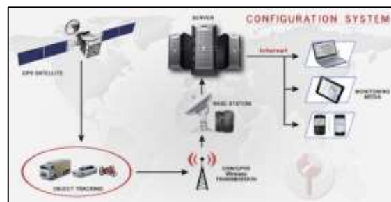
Figure 2 GPS tracker working system
