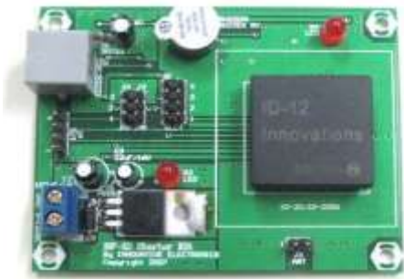
Gambar 2 Reader RFID stater kit ID-12 LA.
