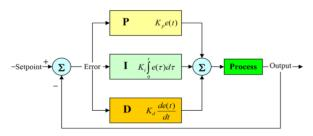
Fig. 3 Block diagram of PID Controller
