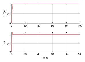
Fig. 5 Responses of Surge and Roll Motion by PID Control System
