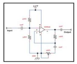
Figure 3.1 The signal-sensing Pre-AMP series
