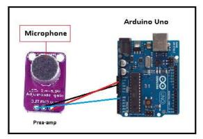
Figure 3 .4 Microphone circuit wiring test
