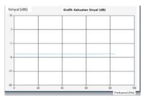
Figure 3,19 Images of signal strength test result-7dB at 2000Hz frequency
