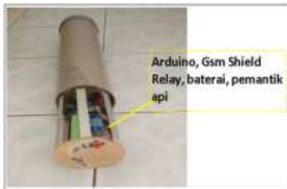
Figure 3.9 Figure of Testing Device for Phone Calls Through an Android Device
