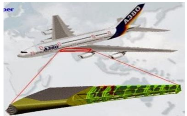
Fig. 3 Inboard outer fixed leading edge part of Airbus A380 manufactured by PT DI
